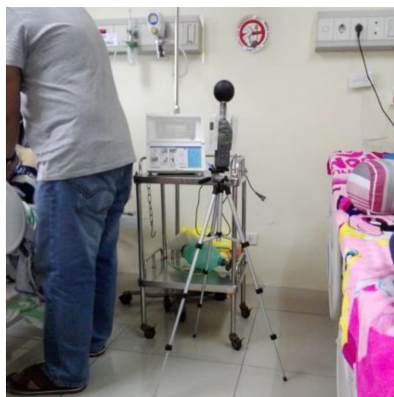
Figure 1. Instrument set-up during field study. Instruments were left to acclimatized for 10 minutes before recording. The sensors were located in-line with patient's head 1.0 meter above the floor. (Photo by the author)
