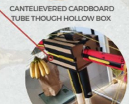
HOLLOW CARDBOARD BOX ACTING AS ATTACHMENT FOR VERTICAL DOUBLE MAST SUPPORT
