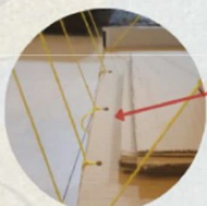
STRINGS TIED TO BASE ACTING AS TENSION CHORDS ATTACHED TO COUNTERWEIGHT SIDE OF CRANE SYSTEM
