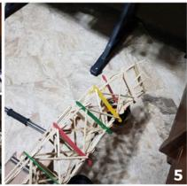
The tie rod was connected to the jib's bottom chord to restrict its tendency to pivot (see "1").
