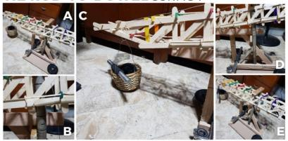
The tie rod was connected to the dowel, the point of load application, contributing significantly to load transfer to the base.
