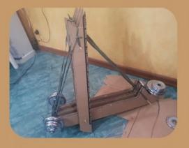
THE STAND COLLAPSED CARRYING 6.60KG LOAD. WITH THE IMBALANCED MODEL AND THE LENGTHY CANTILEVER DISTANCE, THE STAND SLIPPED OUT OF BALANCE TOWARDS THE CANTILEVERED SIDE. WHILE THE COUNTERWEIGHT IS NOT YET CLOSE TO THE LOAD, IT WAS THE EFFECT OF HAVING A LENGTHY CANTILEVER THAT MADE THE WEIGHT IT IS CARRYING MORE CREDIT COMPARED THE ONE CLOSERTO THE CENTER OF MASS.
